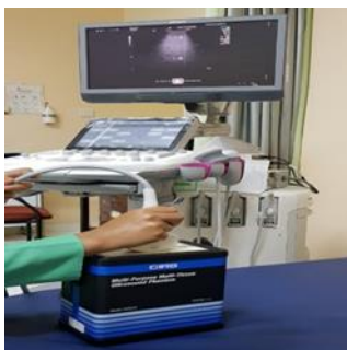
Figure 1. Multi-Purpose Multi-Tissue Ultrasound CIRS Phantom Model 040GSE was used to test the image quality on the Siemens Acuson 1000 ultrasound.
