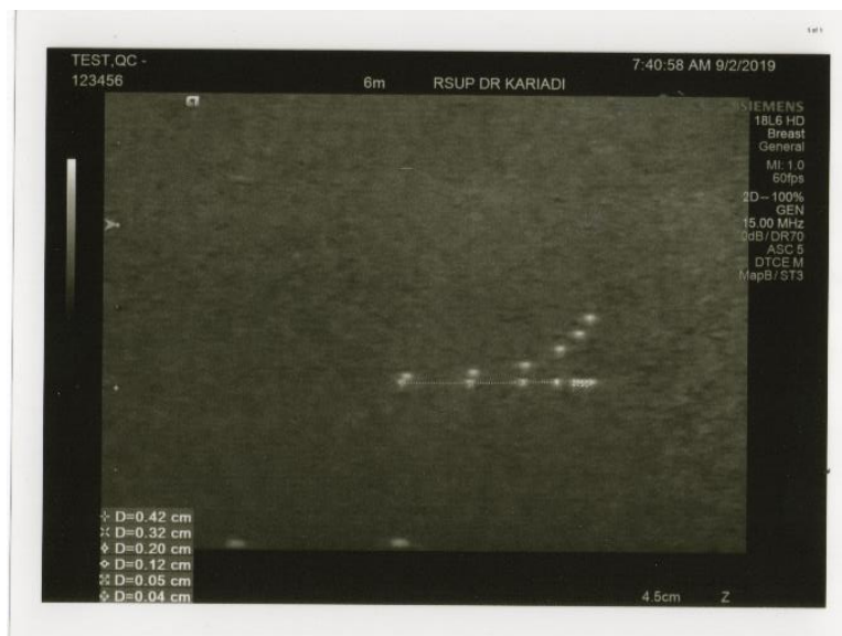
Figure 10. The lateral resolution of the ultrasound quality control using the Multi Purpose Multi-Tissue CIRS Phantom Model 040GSE
