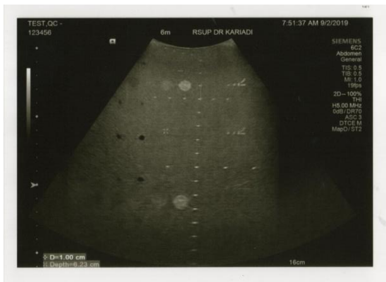
Figure 7. The vertical distance from the Multi Purpose Multi-Tissue CIRS Phantom Model 040GSE
