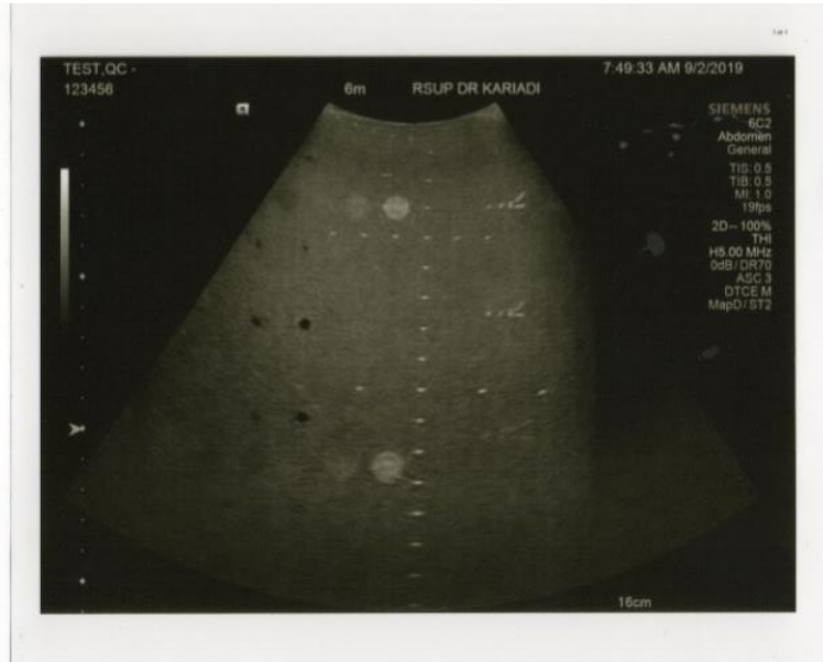
Figure 5. Depth of penetration from Multi Purpose Multi-Tissue CIRS Phantom Model 040GSE
