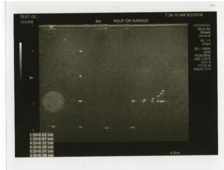
Figure 9. The axial resolution of the ultrasound quality control using the Multi Purpose Multi-Tissue CIRS Phantom Model 040GSE
