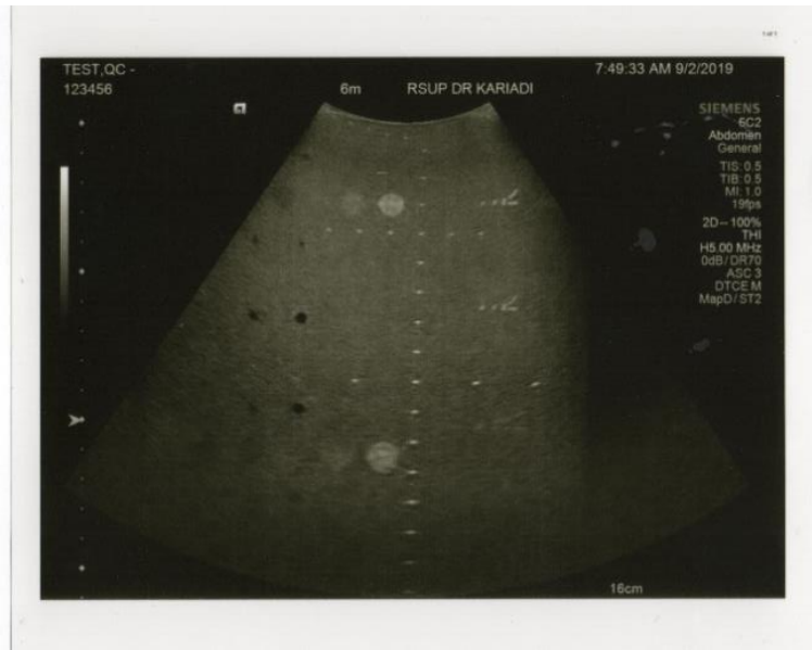
Figure 3. The uniformity of the ultrasound image quality control
