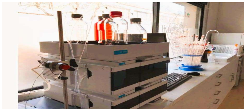
Fig 2: Quality Control and Standardization High-Performance Liquid Chromatography
