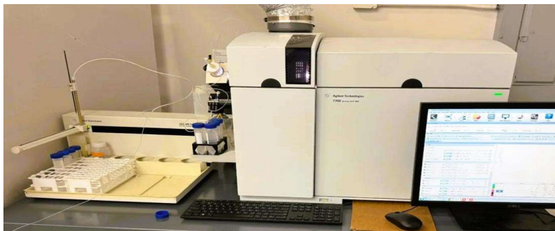
Fig 4: Toxic metal contamination using Inductively Coupled Plasma Mass Spectrometry (ICP-MS)
