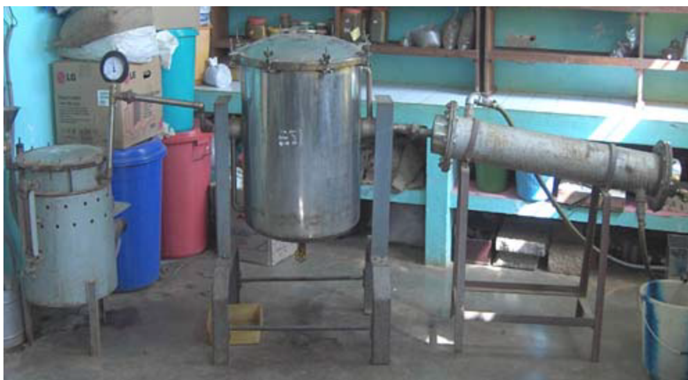
Fig 7: Pilot-scale patchouli steam distillation unit
